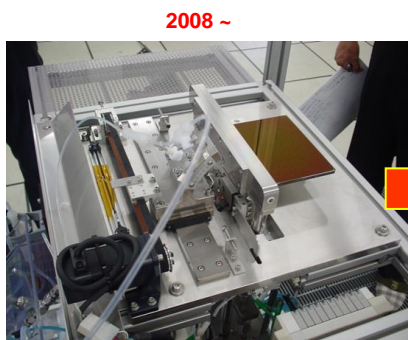
Single slit nozzle & Single type of solvent nozzle 25 minutes/plate
